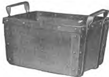
Fig. 205. Wire Basket for Immersing Work in Oil Bath
